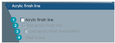
Acrylic finish line: Adds a default 1 mm notch to the bar side. This notch marks the limit for the acrylic finish.
